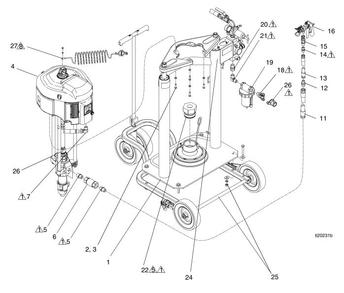
$\triangle$  Apply sealant (8) to all non-swiveling pipe threads.
